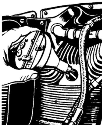
Screw Time-Rite tightly into the front spark plug bushing of No. 1 cylinder after making sure that the piston is on the compression stroke and not too near the top. The Time-Rite cannot be readily installed with the piston at the top of the stroke. Remove all spark plug gaskets.
