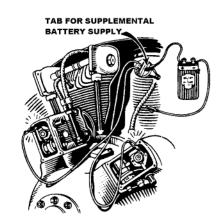
When using Time-Rite for this purpose, it is important to disconnect or insulate the primary coil leads, as is done with any other similar direct current circuit checks on magneto operated ignition systems. The individual magneto manufacturer's recommendation on insulation or disconnection of the primary coil leads should be followed. This is not necessary on battery operated ignition systems.
